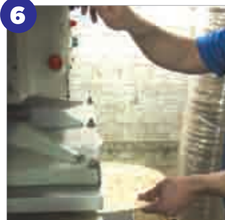
Wood parts are cut on the die cutter to make the seat components.
